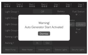
4. The system will attempt to start the generator 3 times. If it fails to start after the third attempt, the system will turn off the Auto feature and display Check Generator fault.
