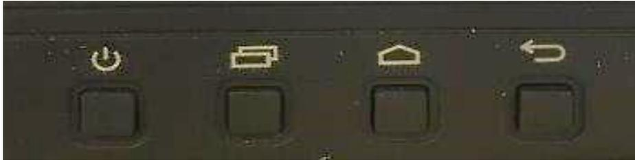
The DC has 4 physical buttons underneath the LCD Display. These are (from left to right) the Power, Pages, Home, and Return buttons. To power on or off the DC, hold the Power button down for 5 seconds. Touch the power button, and the DC will activate (if powered on). The Pages button will cycle the pages on the DC; from Home, to the Functions page, to the Menu page. The Return button will take you to the previous page.
