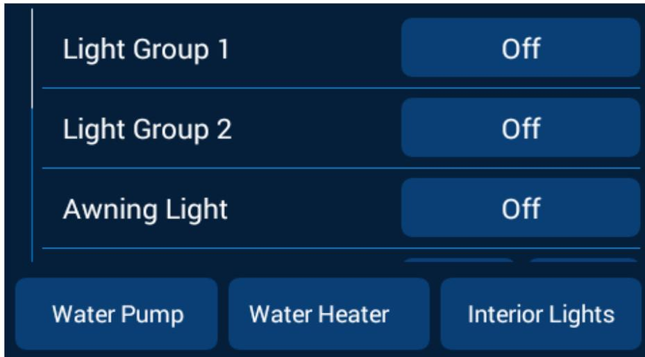
Press the Pages button and observe the Functions Page. Here all the available functions for the RV will be listed. Cycle each function and ensure it works smoothly and corresponds to the correct device. Ensure all the Home Screen "Hotkeys" actuate/turn on the corresponding devices.
