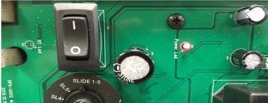
The toggle switch on the BCM corresponds to the dial underneath it. (In the event where communication between the DC and BCM is lost or the DC is damaged, this switch will enable "manual" functions of the selected devices) The switch and knob are used for Motors 1-5 (which could include slide outs, and awnings)
