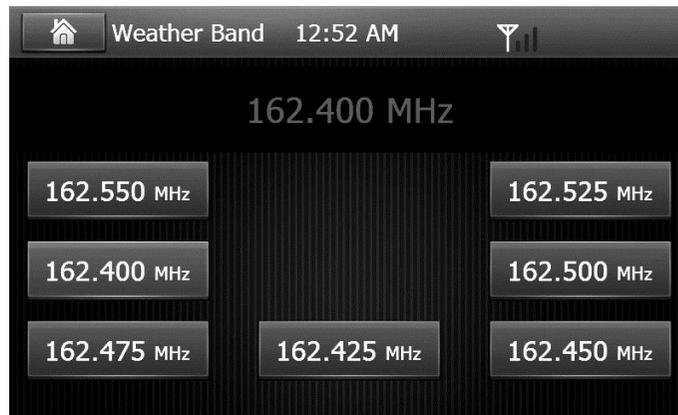
**NOTE:** *The weather band channel frequency is fixed in preset memory and cannot be changed.*
