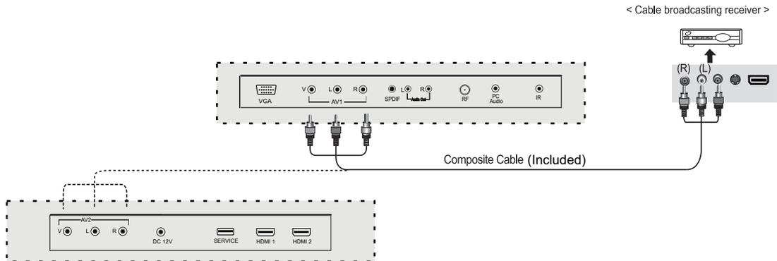
Connect the LED TV's Composite In terminal to the cable broadcasting receiver Composite Out terminal using the Composite cable. (Make sure the color of the terminals and the color of cable are the same)
