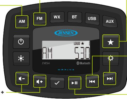
**STATION STORE PRESETS:** Press to cycle through 12 presets channel. Press and hold to access presets store menu, press repeated cycles through 1-12 preset channels, when desired preset slot is selected, press ✓ to store current channel. NOTE: Up to 12 FM & 12 AM channel can be stored.
