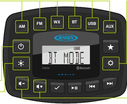
**AUDIO/SETTINGS:** Press to bring up AUDIO ADJUSTMENT options: BASS, TREBLE, BALANCE (left to right), FADE (front to rear), & Loudness (ON/OFF). Hold to bring up SETTING MENU options: BLUETOOTH Device List, BLUETOOTH PAIR, DIMMING (ON/OFF), DIMMING LEVEL, REGION (USA/EURO), PRESET VOLUME and RESET. Press ◀▶ and ▶▶ buttons to select each SETTING option except 'RESET'.
