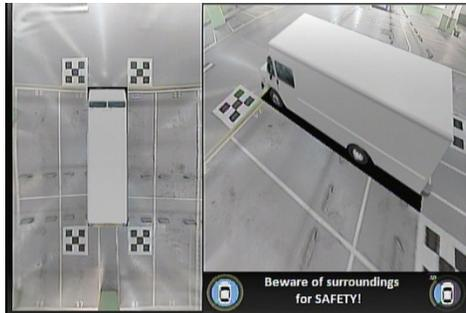
If the Right Turn Signal is triggered, the VAVSMOD2 will give the driver a top view and Right-side view
