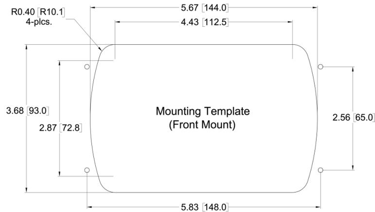
2. Check the dashboard opening size by sliding the radio into it. If the opening is not large enough, carefully cut or file as necessary until the radio slides into the opening. Check that there will be sufficient space behind the dashboard for the radio chassis.
