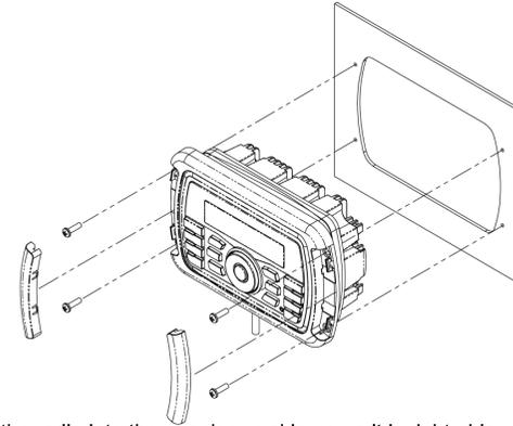
6. Carefully slide the radio into the opening, making sure it is right-side-up.
