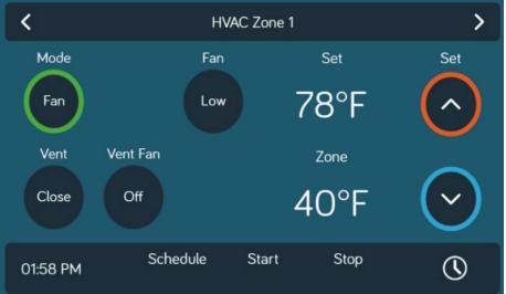
Use the "Set" temperature up and down arrows to set the desired temperature. The "Set" temperature can be adjusted between 55 to 90F.
