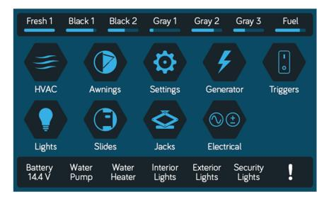
Go through all the functions and make sure they are operating properly. All the functions should be smooth and instantaneous. Ensure all the Home Page Hot keys actuate/turn on the corresponding functions.
