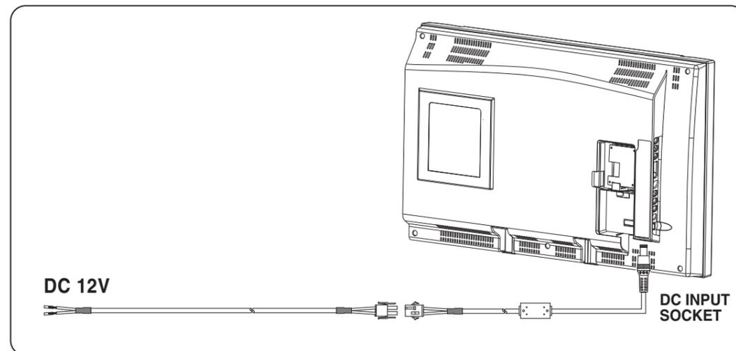
**ATTENTION:** Ensure the power supply is connected to the unit. When not using unit for a long period of time, remove DC input socket from the main power point.
