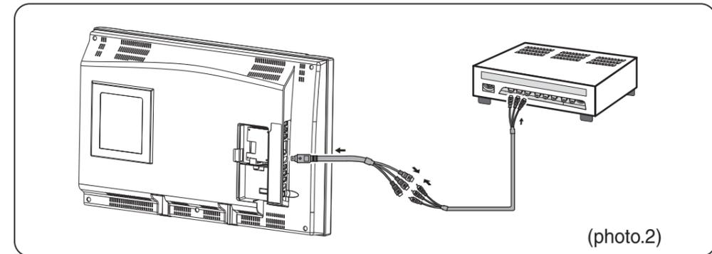
*Noted: When connect Component Video input, please set OSD (AV1 Select) to "CV" to view Component-Video source.*
