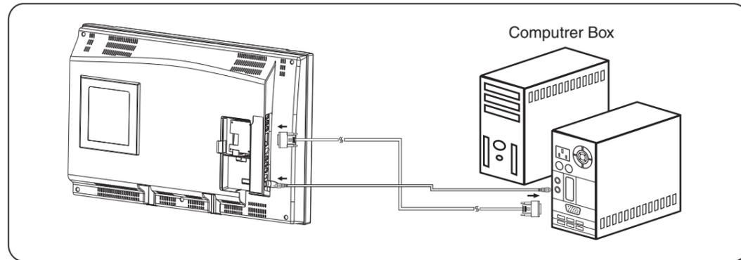
*Noted: When connect VGA input, please set OSD (AV1 Select) to "PC" to view VGA source.*
