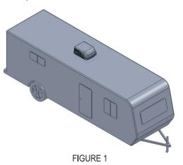
2. For two unit installation: Install one air conditioner 1/3 distance and the other air conditioner 2/3's from front of RV and centered from side to side. See FIG. 2.
