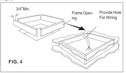
5. The 14-1/4" x 14-1/4"(±1/8) roof opening is part of the return air duct and must be finished in accordance with NFPA standard 501C, Standard for Recreational Vehicles, Section 2-7.
