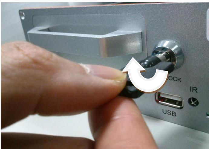
After you installed the SSD, please put the rack back into the mobile DVR, tighten the two front screws and lock the rack. If the lock is not correctly done, the system won't be started up and the power led will flash.
