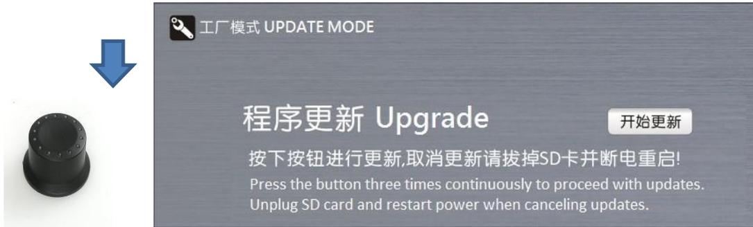
7.5 Keep on pressing the control knob button until you see the window as below. This means the update is processing, please wait for 5 minutes to complete.
