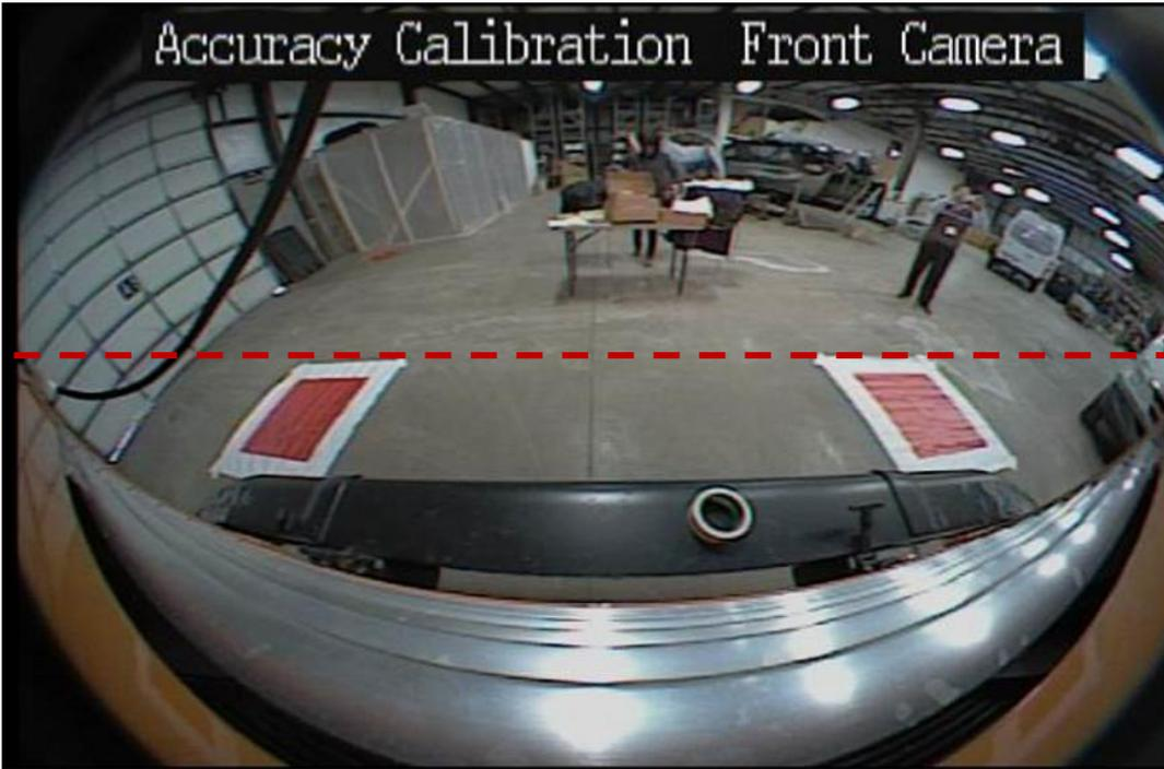
5.3 To acquire photo snapshots, press the control knob once and the snapshot will be saved in SD card once the countdown is complete. The snapshots are saved to SD Card, named as H\_front1000.bmp、 H\_right1000.bmp、 H\_back1000.bmp、 H\_left1000.bmp, shown as below.
