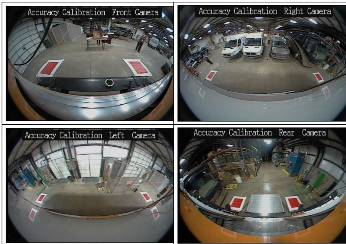
5.2 The Calibration Mats need to be at same horizontal with the top of the Mats in the center of the Monitor Screen. Adjust the camera angle and position Mats are in the proper location on the Monitor Screen.
