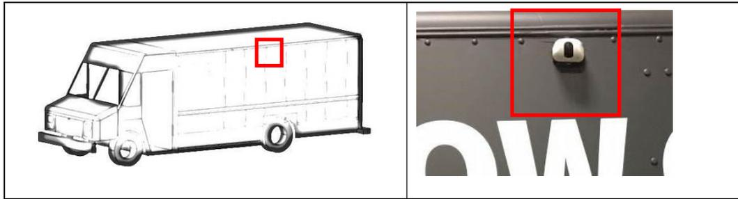
4.4 Rear camera: center of the rear, shown as below. Keep in mind the flatness and the vertical of the vehicle to keep the camera straight.
