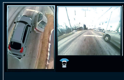
Right-rear corner generated view with front camera view.
