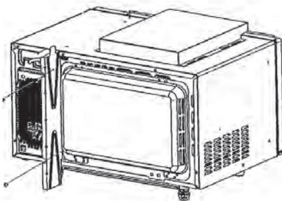
Step 1: Install the top air guide.
