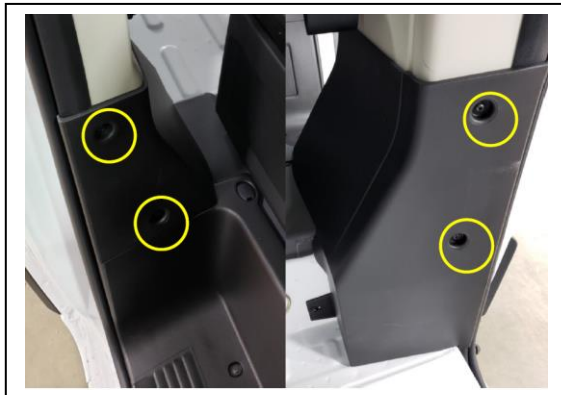
Step 1: Remove B Pillar floor panel on passenger side
