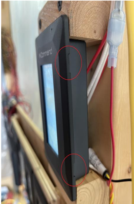
Side View – showing where to pull to remove trim ring
