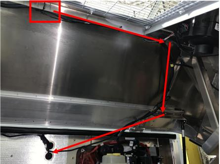
Main module location: Is above the driver's head mounted on the outside as shown or inside
