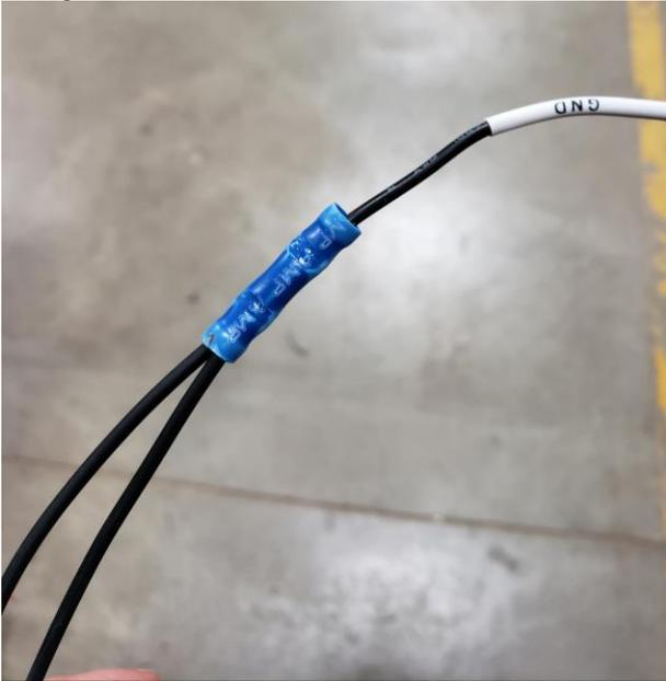
6. Un-tape the Black, Yellow, Green, and White/Red wires on the Connector shown below. Connect the Yellow Wire to the Battery White/Red wire; use the Blue Butt Connector supplied.
