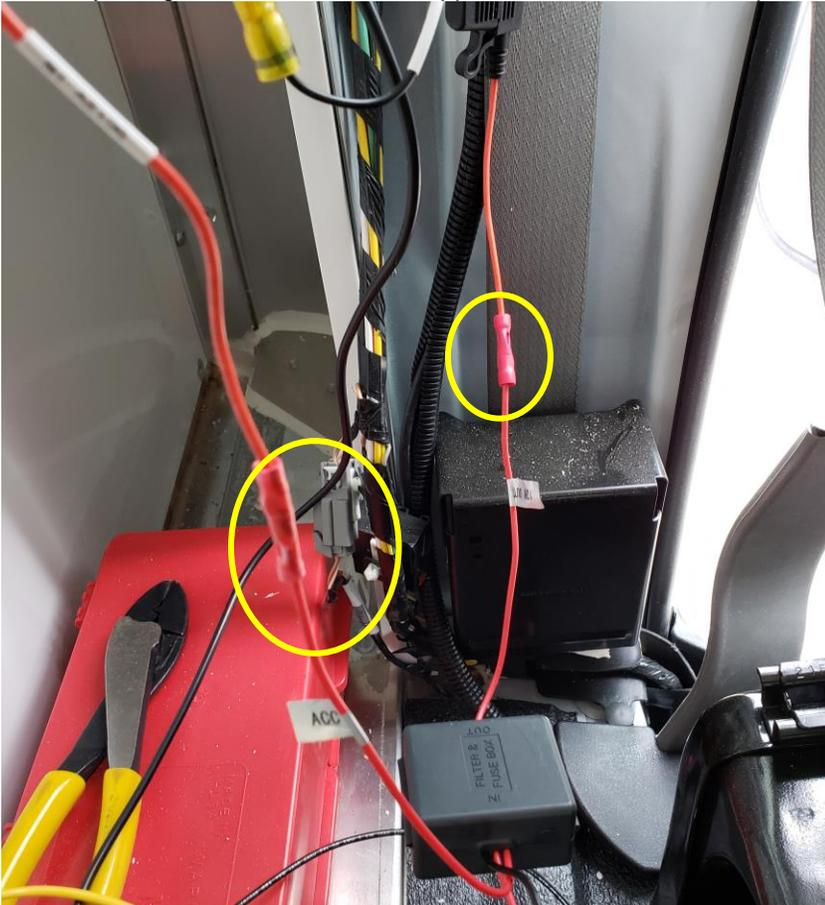
5. Using the Blue Butt Connector, connect the Field Fix Ground Wire with Monitor Ground Wire:
