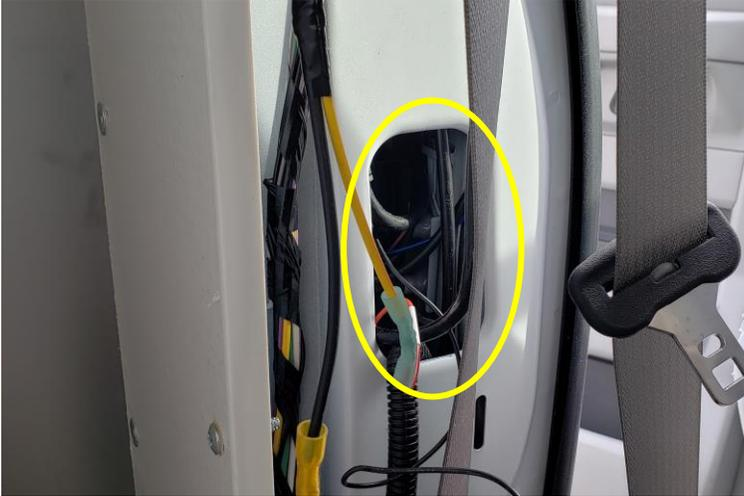
2. To access the Harness, remove the Driver's B-pillar cover by removing the 1/4" Socket Head screws shown below:
