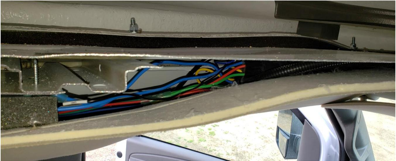
2. To access the Harness, remove the Driver's side shelf panel by removing the screws shown below:
