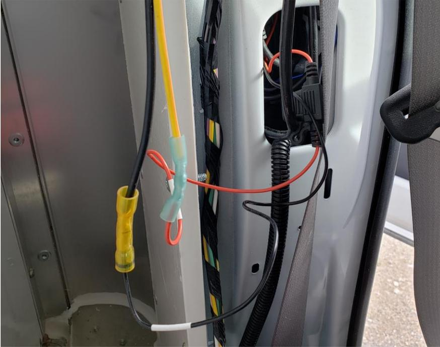
4. To begin inserting the Field Fix Kit, access the DC 12 Volt Wire (Red Wire). Insert the Field Fix Component as shown below by using the Butt Connectors applied to the Field Fix Component:
