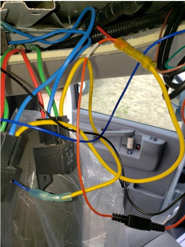
4. To begin inserting the Field Fix Kit, access the DC 12 Volt Wire (Red Wire). Insert the Field Fix Component as shown below by using the Butt Connectors applied to the Field Fix Component:
