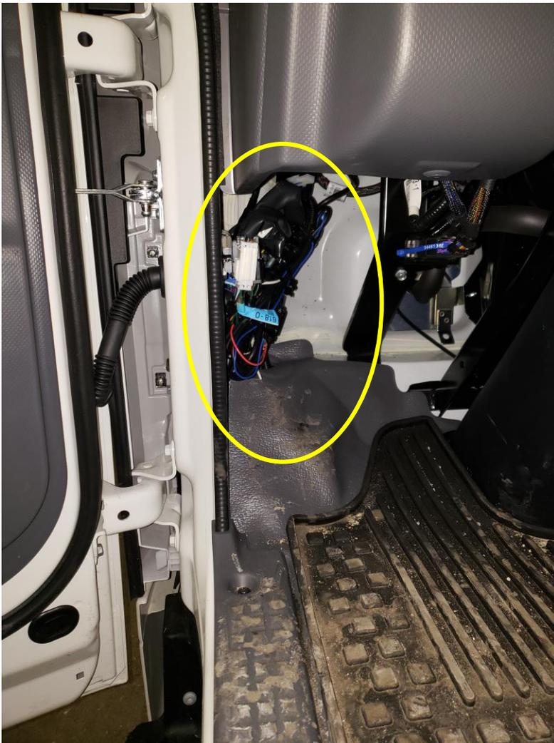
2. Remove the Wire Ties (Zip-Ties) and unravel the Monitor Harness to access the DC 12 Volt Wire (Red Wire):
