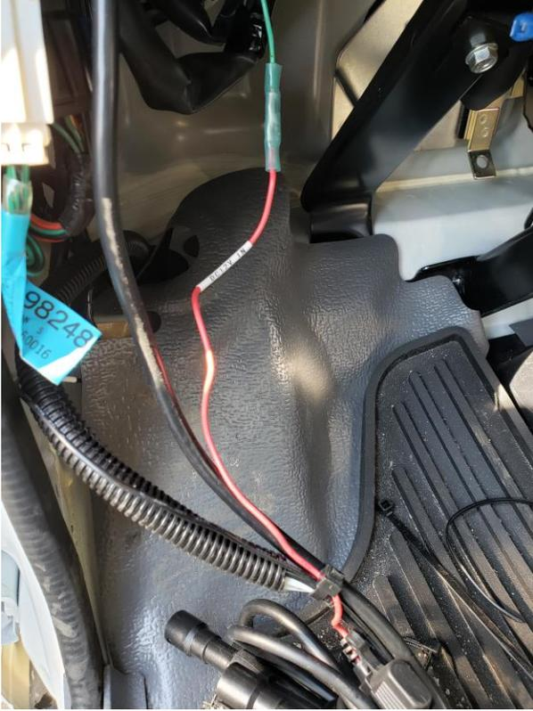
3. Insert the Field Fix Component as shown below by using the Butt Connectors applied to the Field Fix Component:
