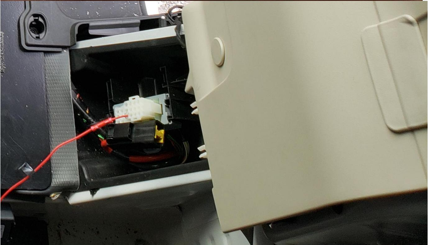
4. Attach the Battery and Ground ring terminals of the relay harness to the Battery Positive Power Terminal and Ground Terminal, respectively. To achieve this, remove the Step Guard via screws; remove caps to access screws;
