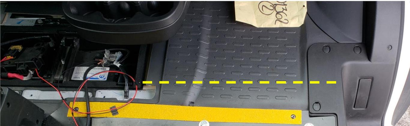
6. Then attach the Battery Ring Terminal to a positive battery power terminal and the Ground Ring Terminal to the Negative Battery Terminal.
