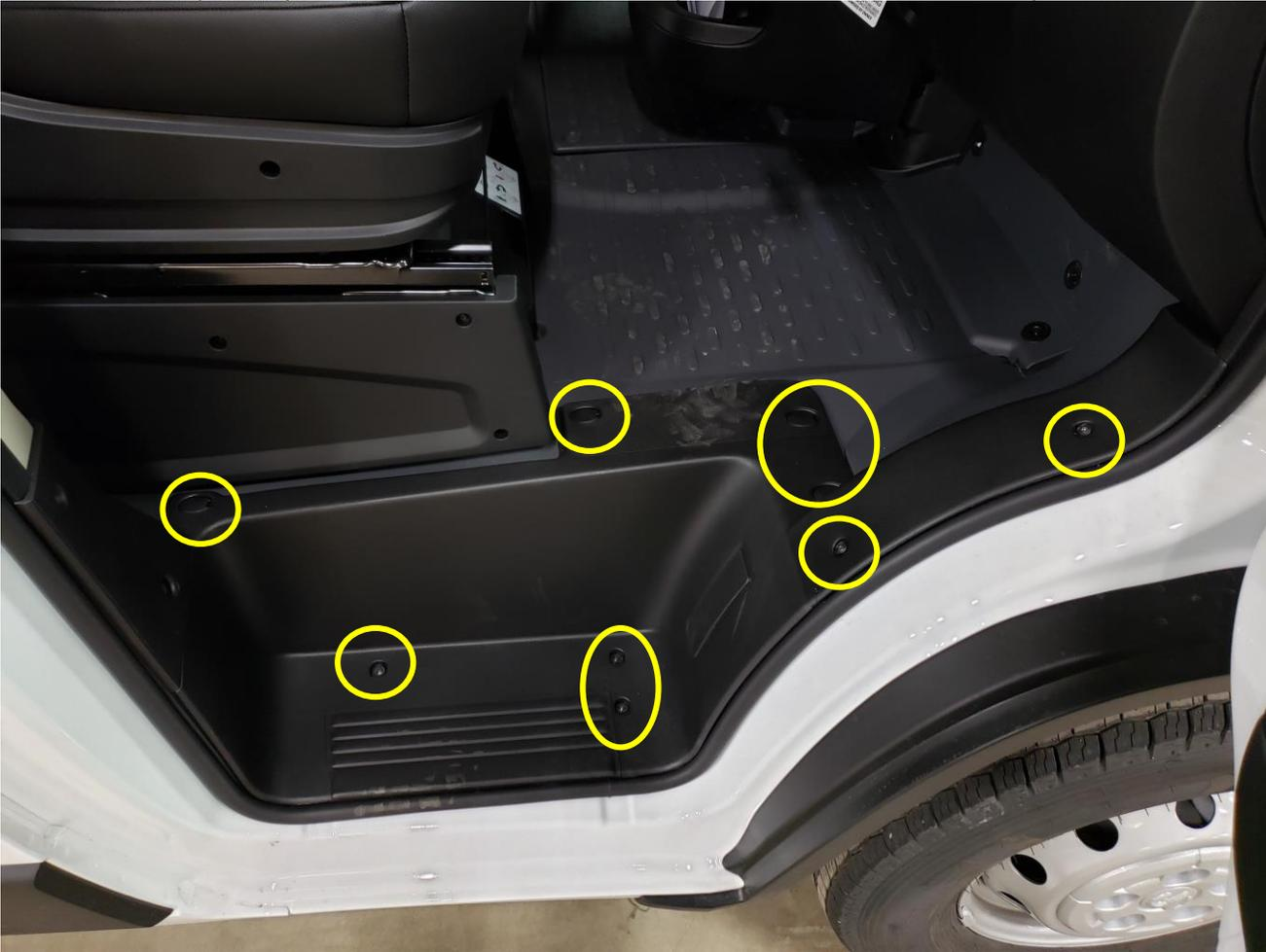
5. With the Step Guard removed, the Harness that contains the Ring Terminals can be snaked under the floor-mat to reach the Batteries.
